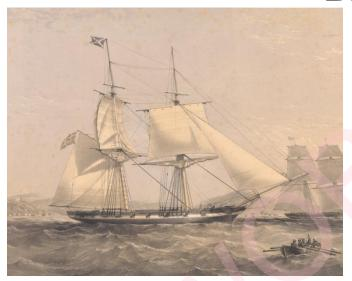
A brig is a type of sailing vessel defined by its rig: two masts which are both square-rigged. Brigs originated in the second half of the 18th century and were a common type of smaller merchant vessel or warship from then until the latter part of the 19th century. In commercial use, they were gradually replaced by fore-and-aft rigged vessels such as schooners, as owners sought to reduce crew costs by having rigs that could be handled by fewer men.
